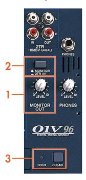
Extra MONITOR functions are found in the [DIO/SETUP] menu, on the MONITOR screen. Different SOLO modes can be chosen, the listening points can be changed (Pre/Post Fader), and the monitor can be switched to MONO:
