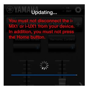
6. The update process takes approximately 30 seconds, and the app will notify you when it has been successfully completed. Following this, disconnect the i-MX1 or i-UX1 from your iOS device and reconnect it. You can then use it with the new firmware.
