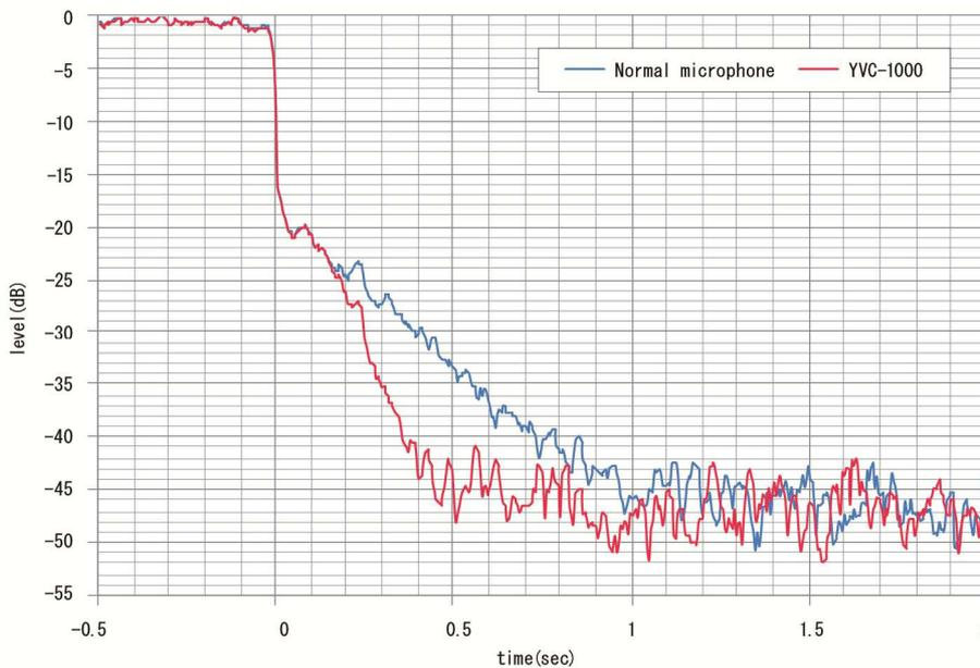
As shown in Graph 2-4, a measuring sound (white noise) was reproduced from a supposed person's location and then the reverberation convergence time from the reproduction stop time (0 sec in the graph) was compared between a normal microphone (without dereverberation) and YVC-1000's microphone. It is clear from the results that YVC-1000's reverberation converges more quickly than the normal microphone's.
