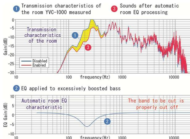
As the graph shows in the shaded in yellow section between ① and ③, it is clear that excessively-boosted bass is
