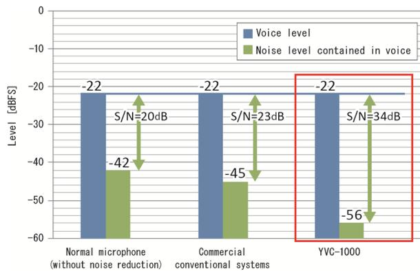
Graph 2-3 indicates the measuring of noise reduction capabilities in environments with background noise levels of 48 dB (air conditioners set to high).
