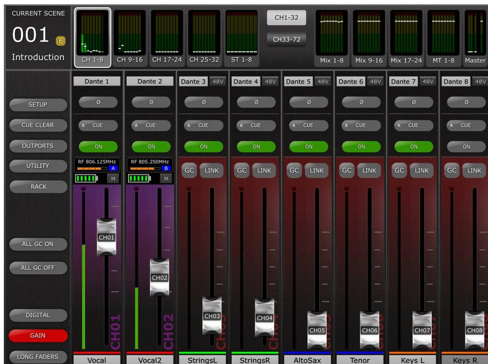
The fader will control the output gain of the wireless receiver(RX) channel. Above the fader, the current battery status of the wireless microphone is displayed. To the right-side of battery indicator, the Mute status of the receiver audio output is shown (if available on the wireless
