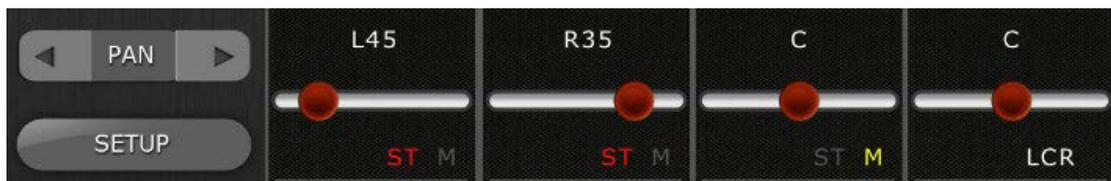
Text shows whether each channel is assigned to the ST, Mono or the LCR busses.
