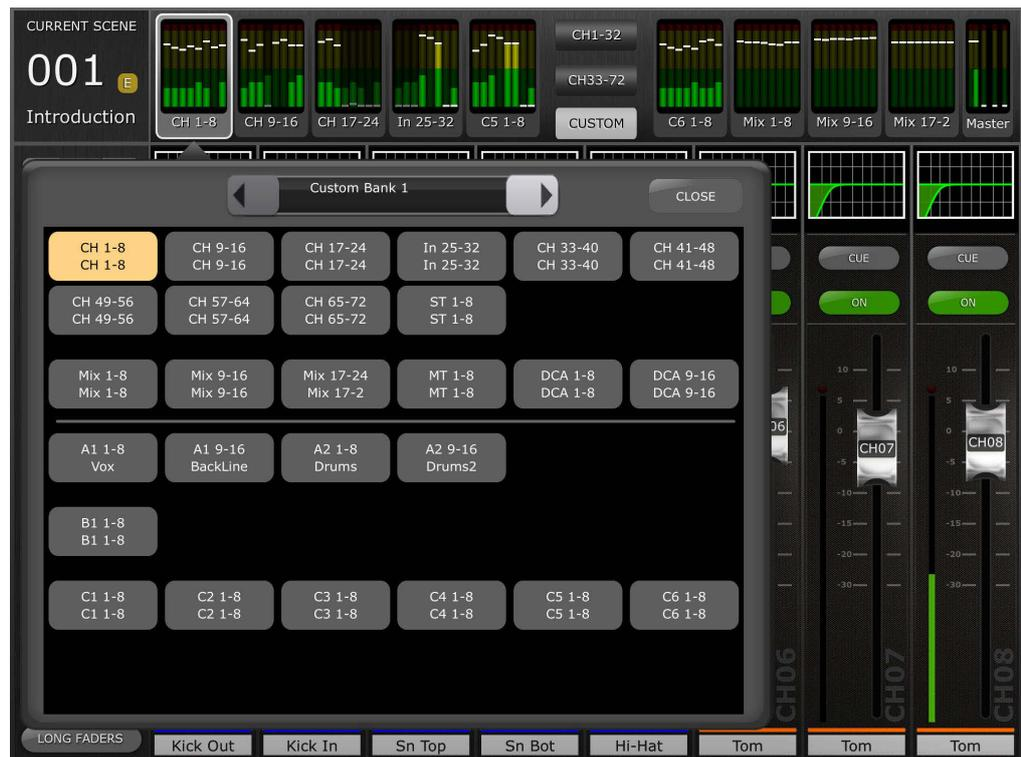
Left/Right navigation buttons can be used to navigate to other meter blocks without leaving the assignment pop-up. To exit the assignment pop-up, touch anywhere outside of the pop-up or touch the close button in the top right corner.
