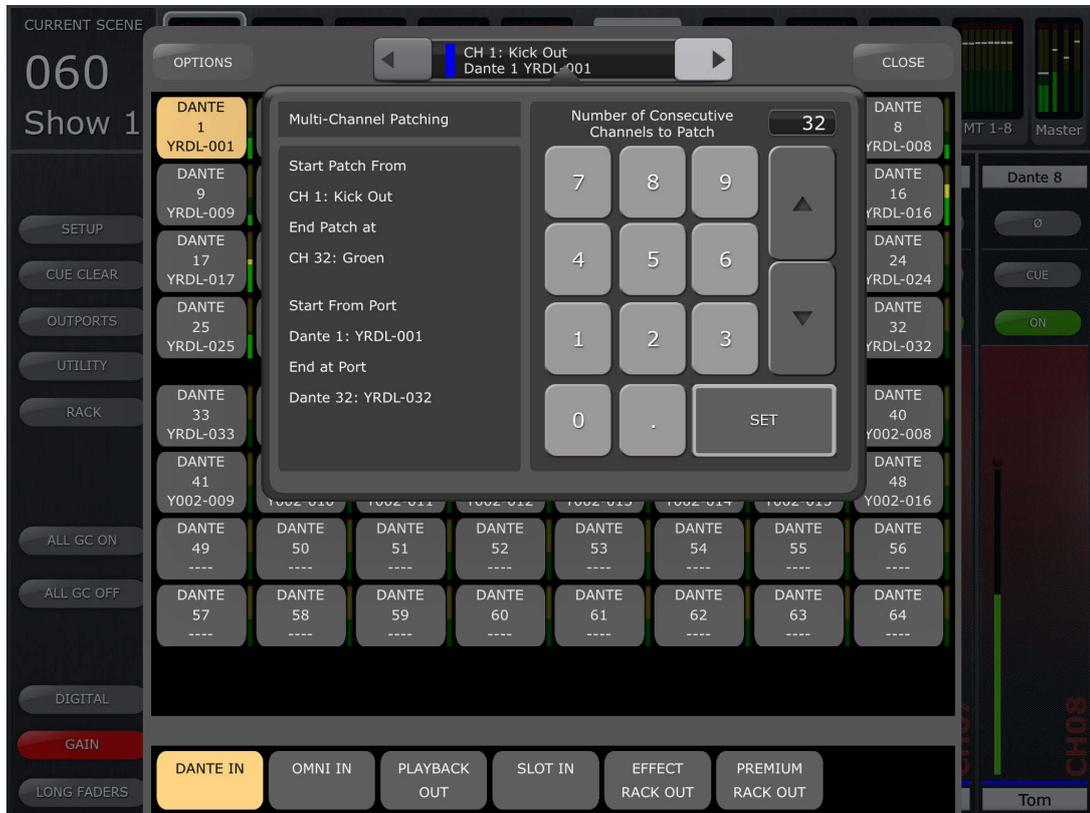
Using the keypad, enter the required number of consecutive channels to be patched. On the left-side of the popup, the start and end channel for the multi-channel patch will be displayed, along with the start input port and the end input port. Touch [SET] to perform the patch and a confirmation message will be show, which outlines the total patch operation which will be performed. Touch YES to continue with the Multi-Channel Patch, or NO to return to the Multi-Patch popup.
