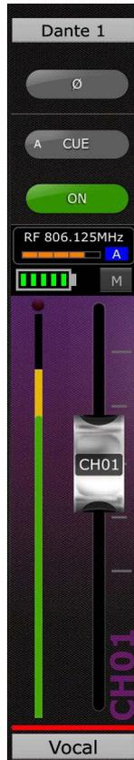
Above the battery and mute indicators, is the RF Intensity meter and the diversity A/B indication.
