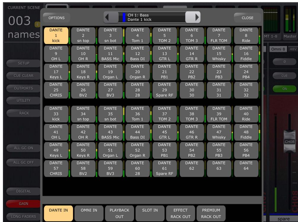
The selected channel number and name is displayed in the top line of the window at the top of the view. Underneath this, is the currently applied input port.
