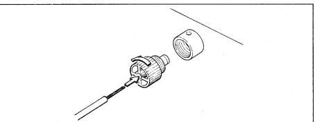
Splay the strands as shown, then screw the wire holders back
