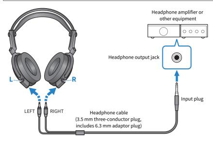
Firmly plug the included headphone cable all the way into the headphone output jack on the device to which you want to connect.
