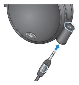
Make sure that the correct cable plugs, L (left) and R (right) are plugged into the correct sides on the headphones, and firmly insert the plugs all the way into the cable jacks.
