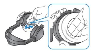
There are four protrusions that fasten the earpad onto the housing, as shown in the following illustration.
