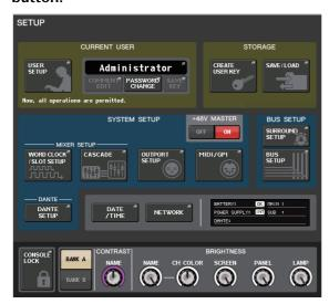
Press the WORD CLOCK/SLOT button in the SYSTEM SETUP field in the middle of the window.
