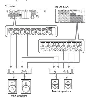
To the OMNI OUT jacks on the CL series and the OUTPUT jacks on the Rio3224-D units, you can patch the output signals from output channels (MIX, MATRIX, STEREO (L/R), MONO (C)), monitor signals (MONITOR OUT L/R/C channels), and the direct out signals of the input channels. For information about patches, refer to "Patching the mixer output to the I/O device" (see page 41) in the Quick Guide section.
