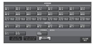
**5.** Return to the previous screen, then press the OUTPUT button in the OSCILLATOR area.
